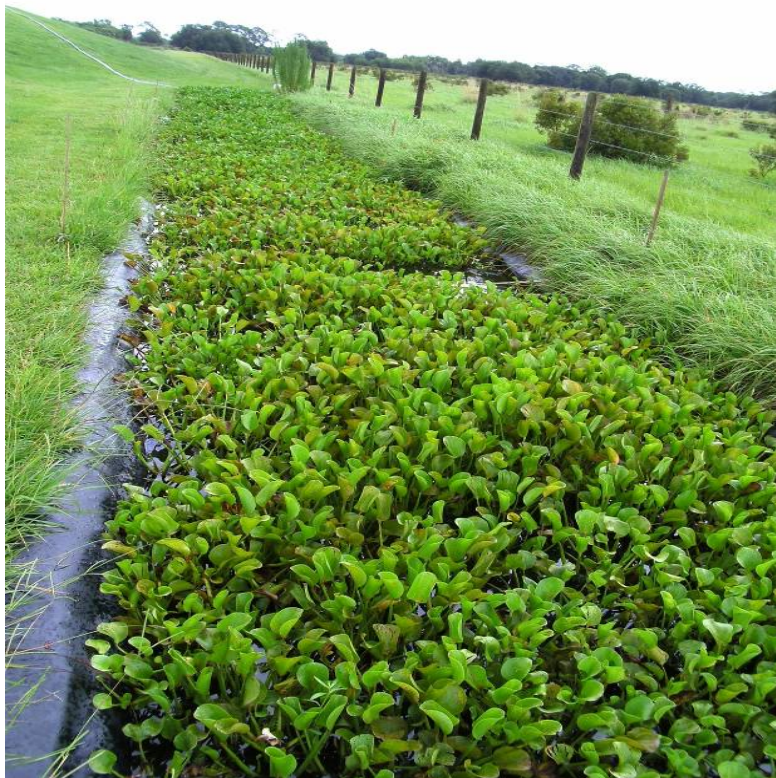
Illustration 18. Water Hyacinth Scrubber (WHS™) pretreatment pilot unit at TC-ATS.
