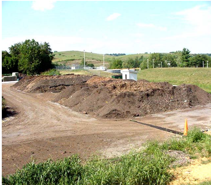
Figure 1. Aerated Static Pile
