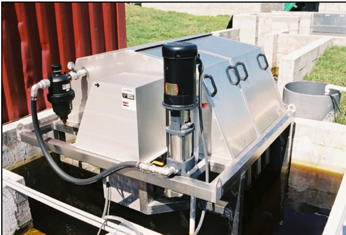
Illustration 10. Hydrotech Model 1704 Discfilter (10 micron)
