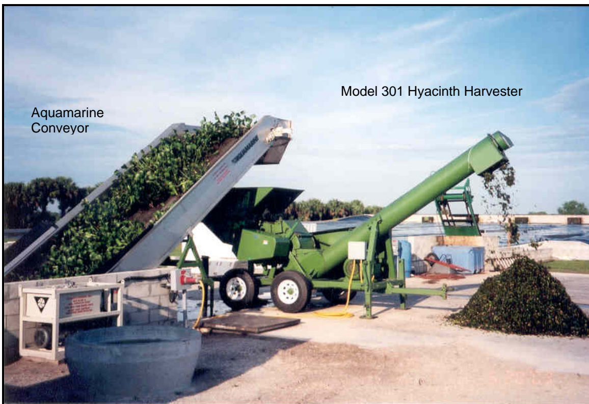
Illustration 6. Hyacinth biomass processing for livestock feed and compost
